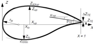
Figure 1 The PARSEC Parameterisation Method
