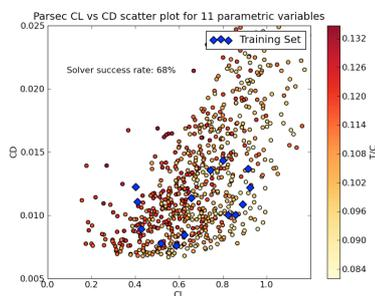
Figure 8 Design Space Generated using PARSEC with 11 Design Variables
