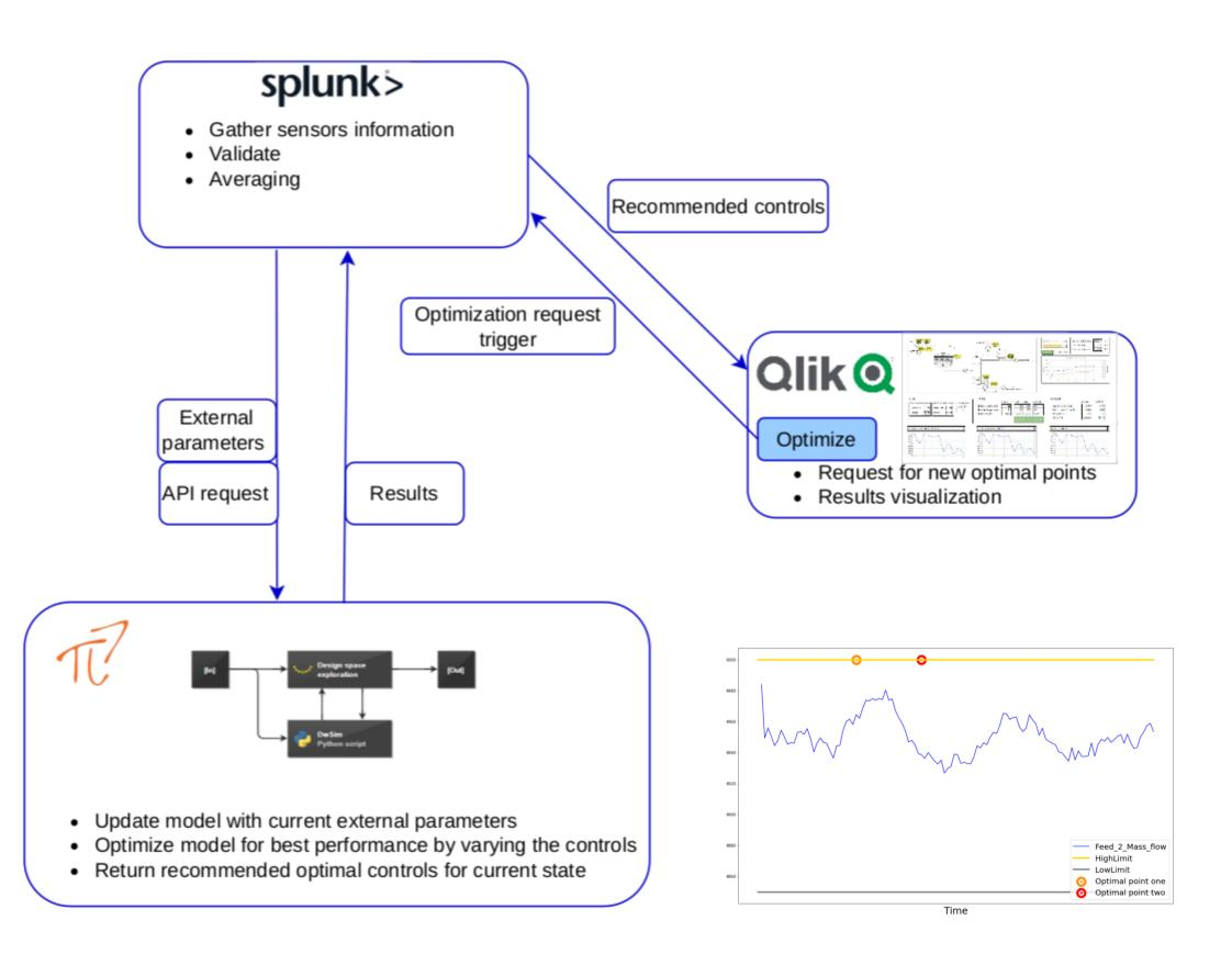
Based on evolving operating conditions (environment like T° in ex. or energy cost), operator can request **unit parameters optimization** based on target function like price margins.
