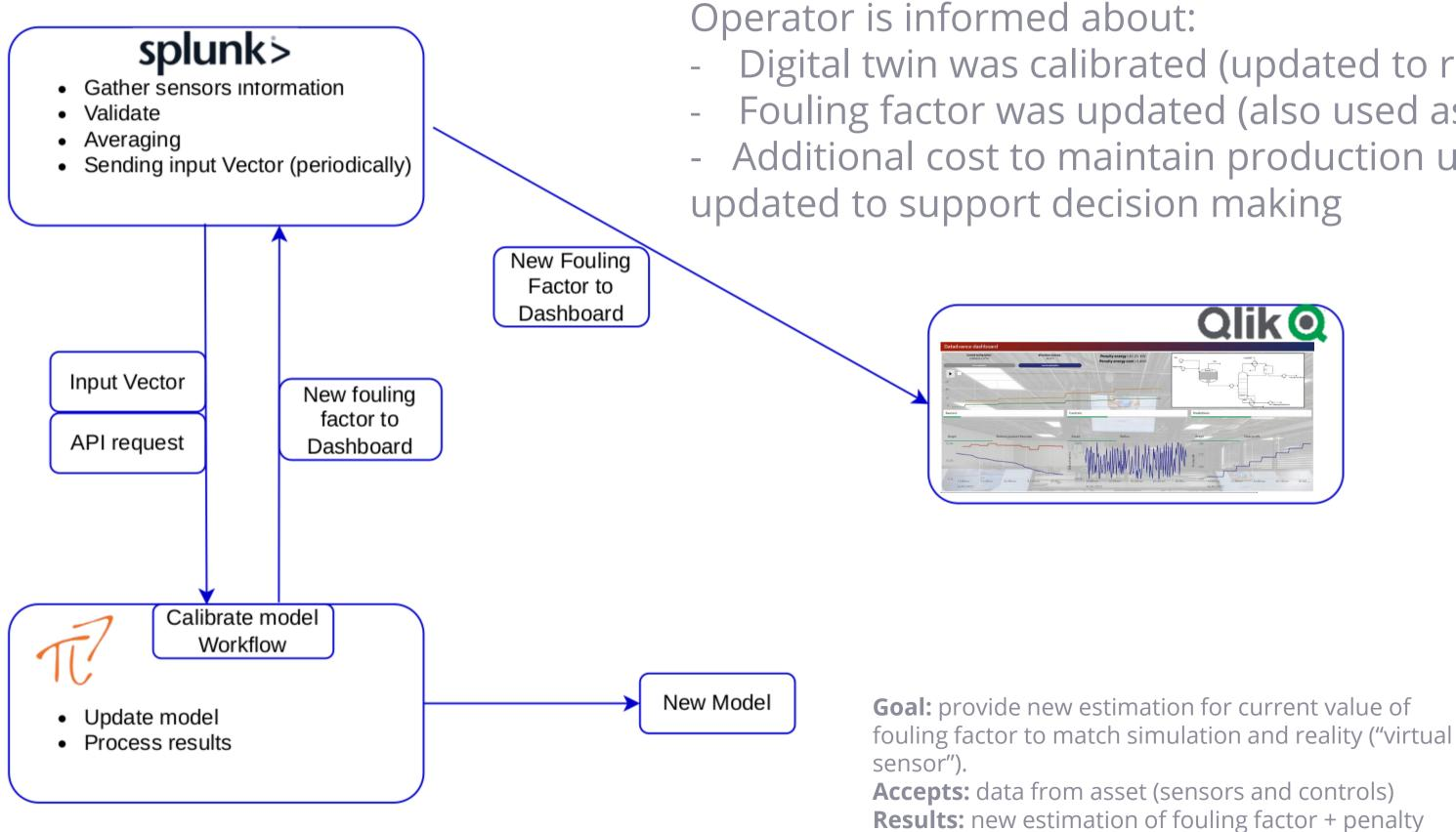
**Accepts:** data from asset (sensors and controls) **Results:** new estimation of fouling factor + penalty energy for new value of fouling factor
