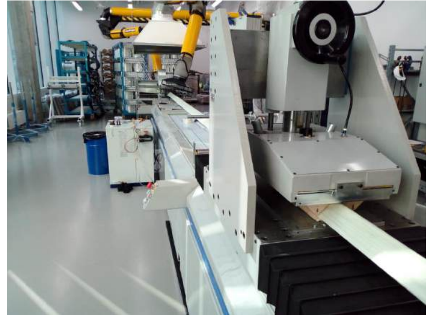
Pultrusion machine: Pultrex Px500-6T
